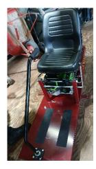
The Club was allocated a grant of \$10,000 from the Brisbane City Council to purchase a new EV battery-operated greens roller thanks to the hard work of our Grants Officer, Tim Salway. The roller has two batteries in operation and two spares that will fully charge in 20 minutes. This gives ample charge to roll both greens with an easy battery changeover if required.
